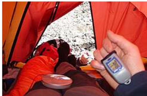
Using an oximeter. This instrument can be a useful indicator of altitude problems
